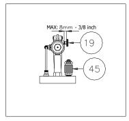
When spraying solvent based products **always** fully close the air regulator (BS45) on top of the tank cap. Close it by turning counter clockwise.
