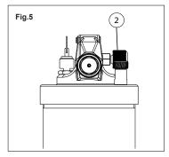
Turning the product control knob (#3) clockwise will gradually reduce the rate of product flow. Turning it counterclockwise will increase the product flow.
