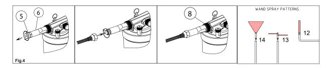
The gun is supplied with wands to spray wax based rustproofing. The wax can be sprayed directly out of the gun or with the wands attached.
