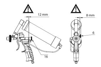
Adjusting the product atomization: Turn the Air Control Knob (PM/2.06) clockwise to close the air passage gradually. This will reduce the atomization and make the texture rougher. Turn the Air Control Knob anticlockwise to increase the atomization and spray a smoother texture.
