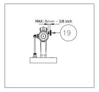
Turning the product control knob (BS09) clockwise will gradually reduce the rate of product flow. Turning it counterclockwise will increase the product flow.
